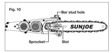
7. Replace the chain/sprocket end cover by positioning the cover onto the saw head. Fit the end cover knob by inserting the bar stud into the bar stud hole. Tighten the end cover knob, but leave the bar free to move for tension adjustment (Fig. 11).
